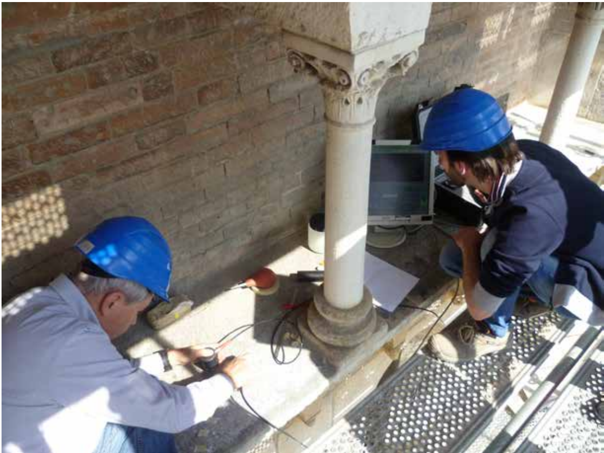
Ghilrandina Tower, diagnostic surveys by ultrasound
